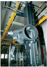
Metal shot-blasted base frame prior to the immersion operation.
