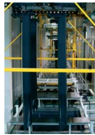
In the individual immersion tanks (13 in number) the crane parts are degreased, washed, activated, coated with zinc phosphate, washed again, de-activated and after rinsing with ultra-clean water they then undergo the electrostatic KTL coating process.
