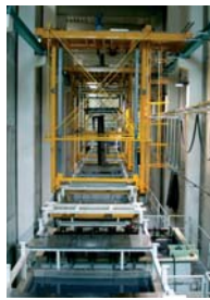
In the individual immersion tanks (13 in number) the crane parts are degreased, washed, activated, coated with zinc phosphate, washed again, de-activated and after rinsing with ultra-clean water they then undergo the electrostatic KTL coating process.
